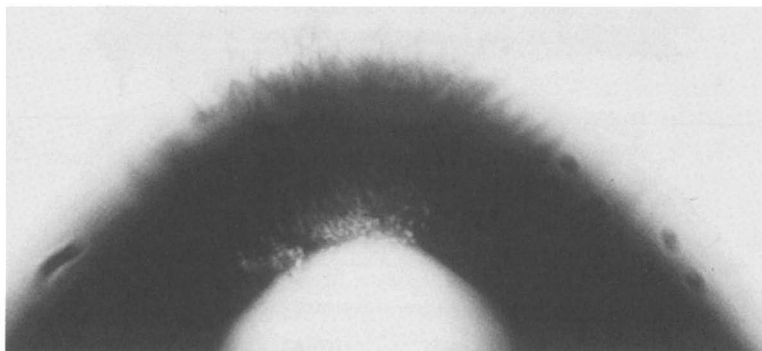
Figure 8. Montmorillonite particles accumulated on the down-stream side of an air bubble. The air bubble was about 300 \mu\text{m} in diameter, and the sizes of particles were \leq 0.5 \mu\text{m} . The photomicrograph was taken under transmitted light.
